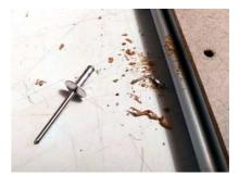
10. Fix the hardboard back to the farme with a riveter.
